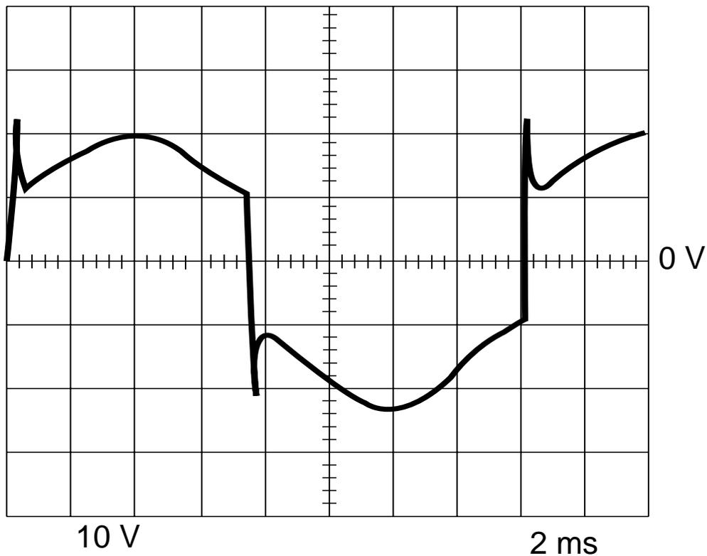
**MACHINE LOADED TO 180 AMPS AT 16VDC.**
