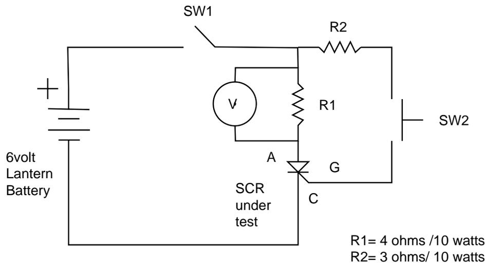
To test SCRs construct the circuit outlined above. Resistor values are plus or minus ten percent. The voltmeter scale should be low, approximately 0-5 or 0-10 volts DC.
