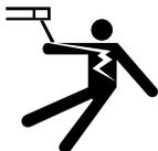
• In Stick Mode the output terminal and electrode will be electrically hot whenever the power switch is turned on.
