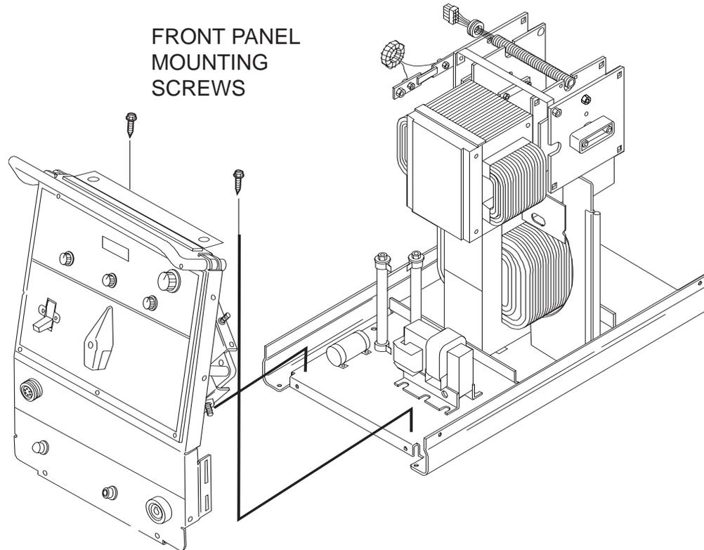
9. Remove plug J2 from the control board. (See **Figure F.9.**) Also remove plug and lead harness from internal divider panel.
