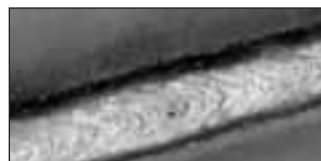
Power Mode aids bead wetting and penetration on aluminum.
