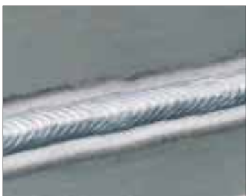
Pulse-On-Pulse on 3 mm Aluminum
