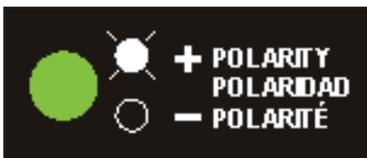
**NOTE:** Both LED's will flash briefly when power is applied to the feeder.
