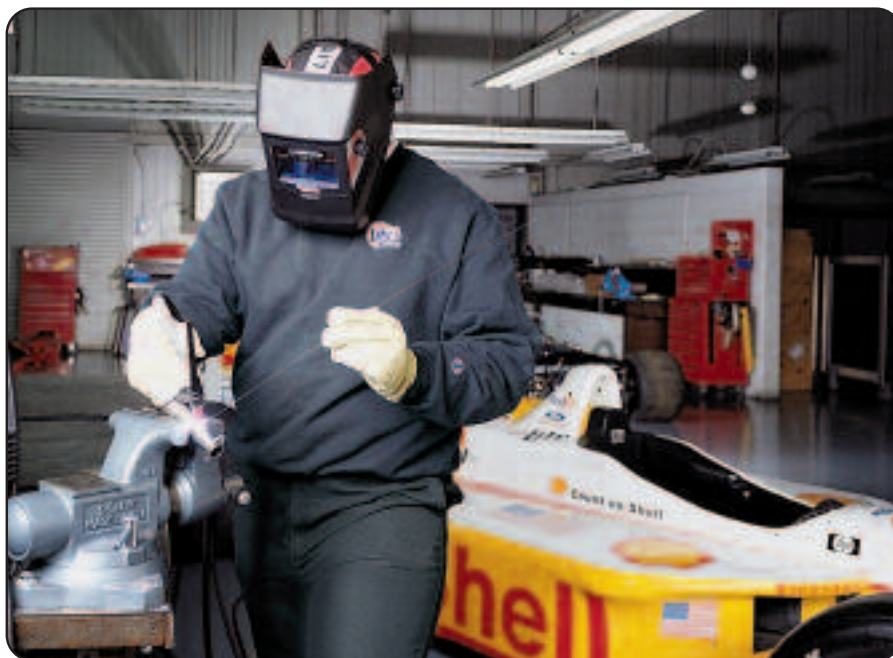
Pulsing capabilities can be used to control heat input on thin materials.
