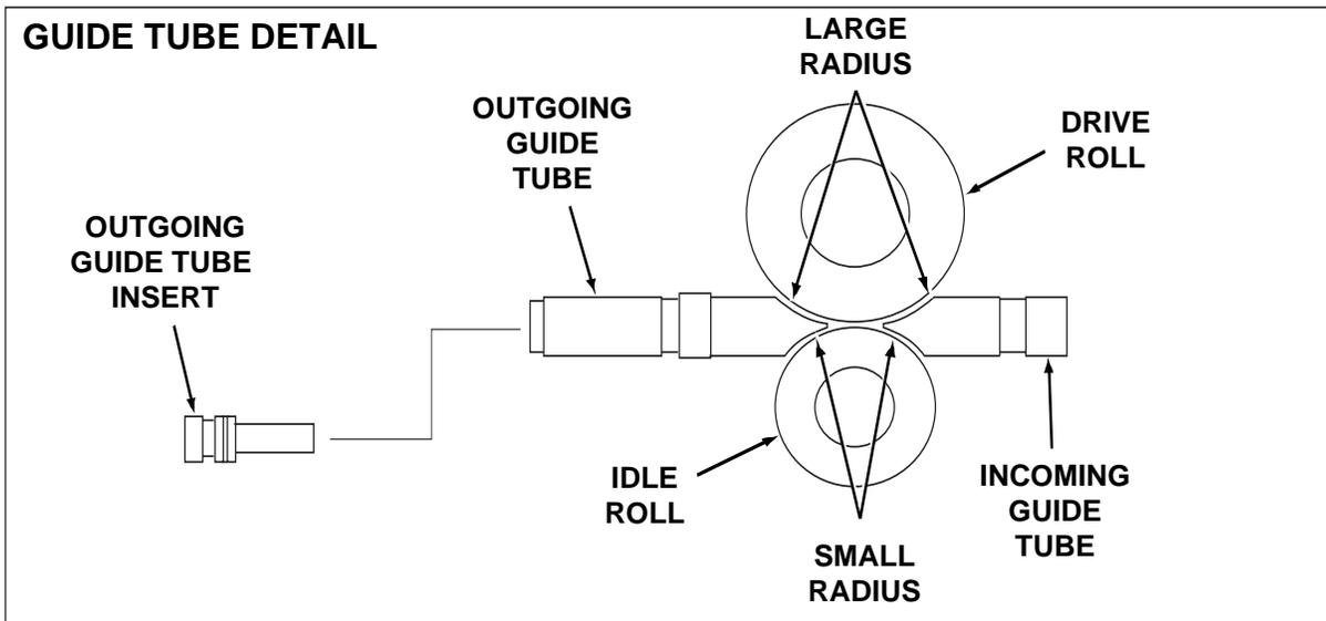
3. Remove the hex head screw and clamping collar. Remove the drive roll from the shaft.
