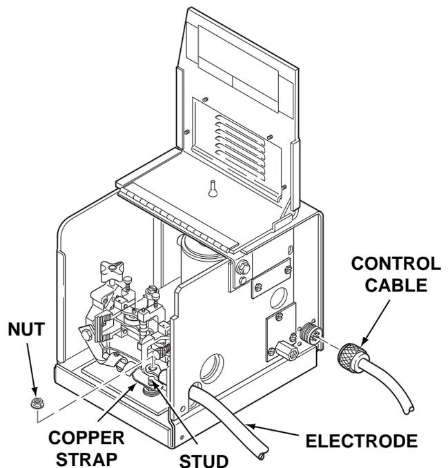
4. Connect the remaining end of the control cable with the eight-socket cable plug to the mating receptacle on the LN-742.
