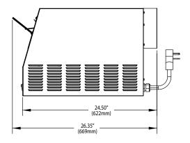
**ELECTRICAL SERVICE**: Heat is supplied by ten (10) infrared heating elements with six (6) on top and four (4) on bottom. Each toaster is rated at 4850 Watts. A separate circuit breaker is required for each toaster. Domestic single phase units require a 30 amp electrical service with receptacle type NEMA 6-30R to mate with a provided NEMA 6-30P plug.
