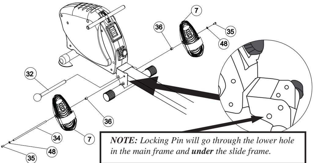
**NOTE:** Locking Pin will go through the lower hole in the main frame and **under** the slide frame.
