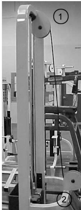
Figure 7. Upper and lower pulleys.
