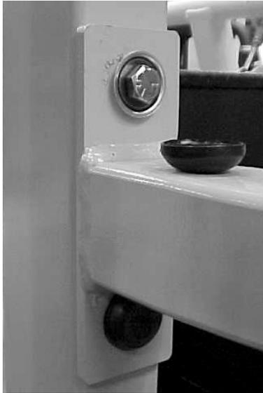
**Figure 4. Bolt (viewed from the Seat Subframe section).**
