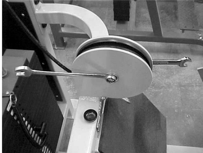
Figure 6. Removing the pulley bolt.
