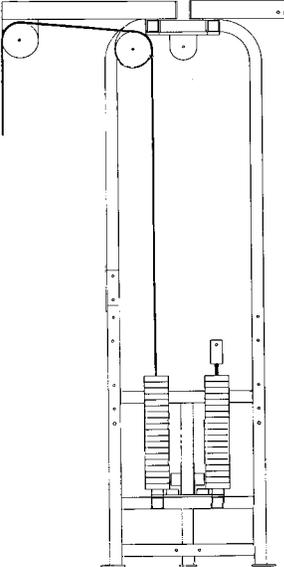
**Figure 19. Tricep pushdown cable routing.**
