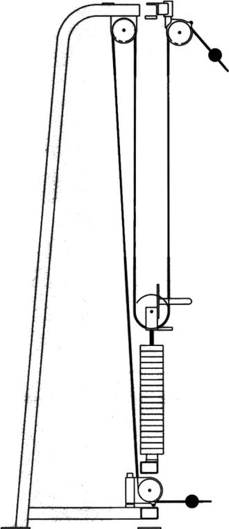
Figure 16. Crossover cable routing.
