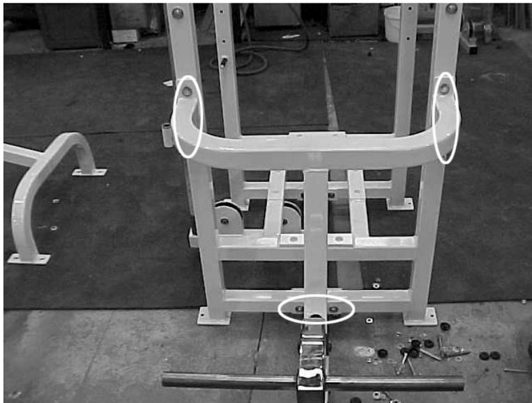
Figure 14. Bolt the bench to the frame.
