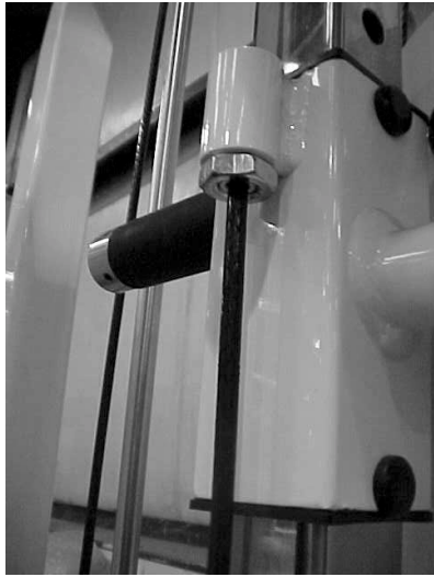
Figure 7. Adjustable crossover cable end detail.
