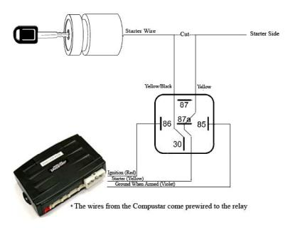
prewired to the starter kill relay. If you are not installing anti grind/starter kill, you do not need to con nect the thin 24 guage green wire.
