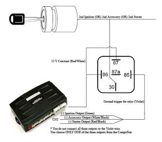
the negative (-) Ignition output from Connector 3, to the short violet wire coming off of the relay, will provide an additional (+) 12V Ignition output from the long blue wire.
