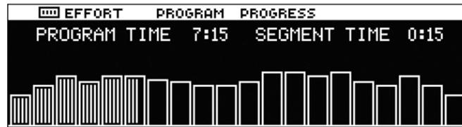
As soon as you begin, the Program Progress screen becomes available. The effort level is shown as 20 bars of a bar graph. The higher the bar, the higher the effort level for that segment will be. Program progress is indicated by the lines that fill in each of the grade segments as they are completed.
