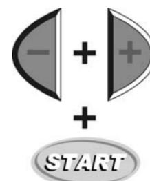
Note: You can also manually initiate the self-diagnostics mode by holding the center “+”, “-”, keys and then pushing **START** when the elliptical is off.
