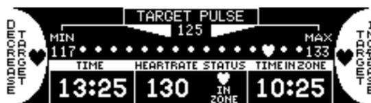
Your target pulse is displayed at the top of the screen. You can adjust this number higher or lower by pressing the center “+/-” keys.
