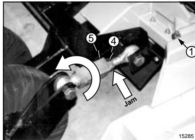
**Wing Leveling Turnbuckle
