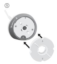
With light pressure turn the transmission disc 4 clockwise, until the resistance yields. The arrows on the transmissiondisc 4 and in the motor unit 3 must point to each other
