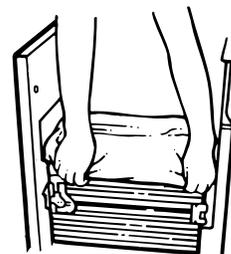
2. Lock bag in place by pulling the four prepunched holes over the bag retainer buttons. Holes will expand over the buttons without damaging the bag.
