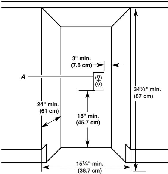
A. Grounded electrical outlet must be a minimum of 3" (7.6 cm) away from surrounding cabinets or nearby walls as shown. It can be placed either to the left or the right side of the compactator.
