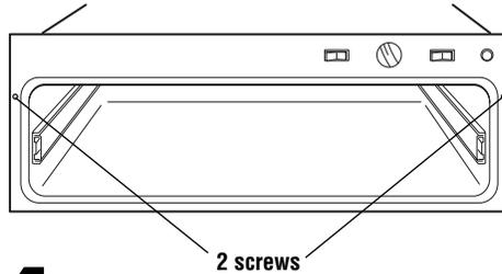
**4.** Use two (2) screws provided to secure the warming oven frame to the cabinet.
