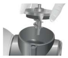
Once the burr-shaft assembly is in the motor housing, rotate the assembly until it falls into place.
