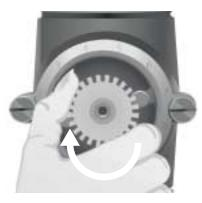
6. When the burrs are touching, turn the grind control gear counterclockwise 1 "click" or detent. The grating or "rubbing" sound will stop. Turn off the mill by flipping the On/Off Switch to the "Off" position. The mill is now calibrated to provide maximum fineness.
