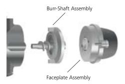
Using the burr-cleaning brush, clean the burr mounted on the burr-shaft assembly and the burr mounted within the motor housing.
