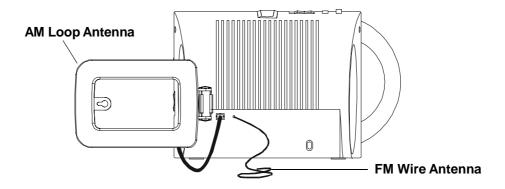
**AM** – Adjust the direction of the AM loop antenna that you connected to the back of the radio. If this does not provide sufficient improvement try removing the loop from the antenna bracket and moving it further away from the radio cabinet (as far as the wire will allow). You may also attach the loop to the wall with a thumbtack or small nail through the "keyhole" on the antenna frame.
