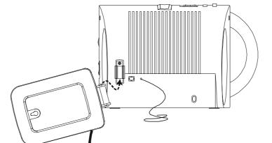
3.) Adjust the angle of the loop antenna until you find the position that provides the best AM reception.
