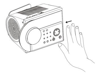
The effective operating range of the Snooze Sensor is approximately 2 inches. The Snooze function will stop the alarm for 5 minutes and then turn the alarm on again. The Snooze operation can be repeated several times within one hour. But after one hour the alarm will not turn on again.
