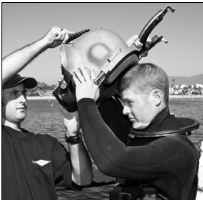
Open the locking collar/neck pad assembly fully.
