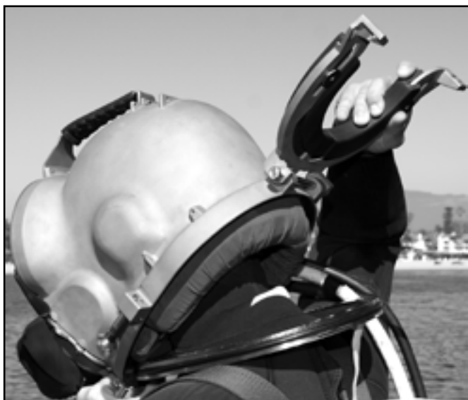
The locking collar must be completely open for the diver to don the helmet.
