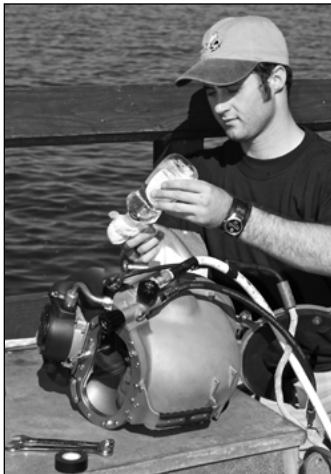
A thin film of dish soap or other anti-fogging solution should be applied to the lens prior to the diver donning the helmet.
