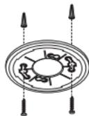
When wall mounting, the "A" line should be horizontal.
