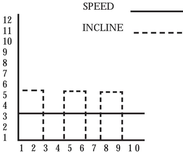
The **Fat Burn Program** is designed to vary the treadmill elevation, while maintaining a constant walking belt speed.
