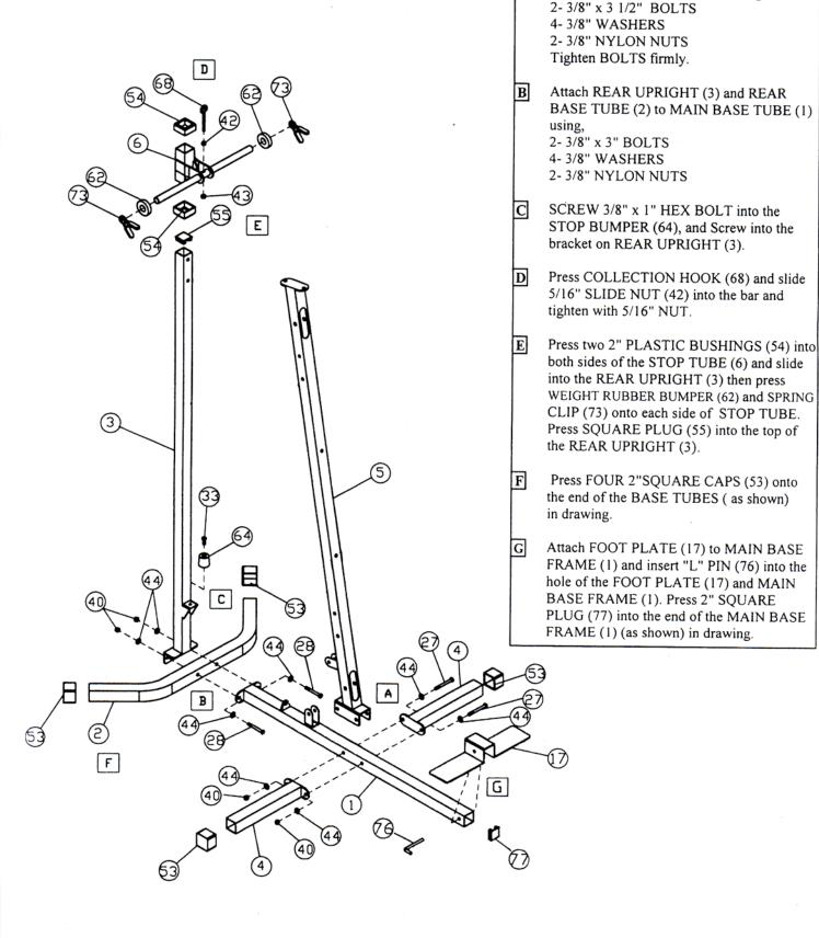
Attach FRONT UPRIGHT (5) and two FRONT BASE TUBES (4) to each side of the MAIN BASE FRAME (1) using,
