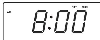
To change the Alarm Mode setting for Alarm 1, hold the **ALARM 1** setting button and press the **ALARM MODE** button until the Day indicators show the desired mode setting, Weekdays only, Weekends only, or Everyday operation.
