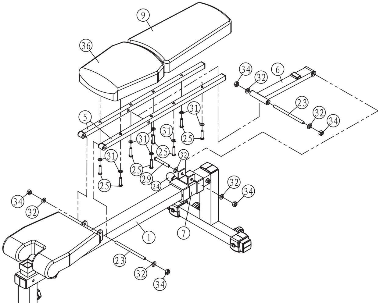
**STEP 3** First attach Back Support Tubes (5) to Main Frame (1) using Screw Shaft (23), Washers (32), and Nylon Lock Nuts (34).
