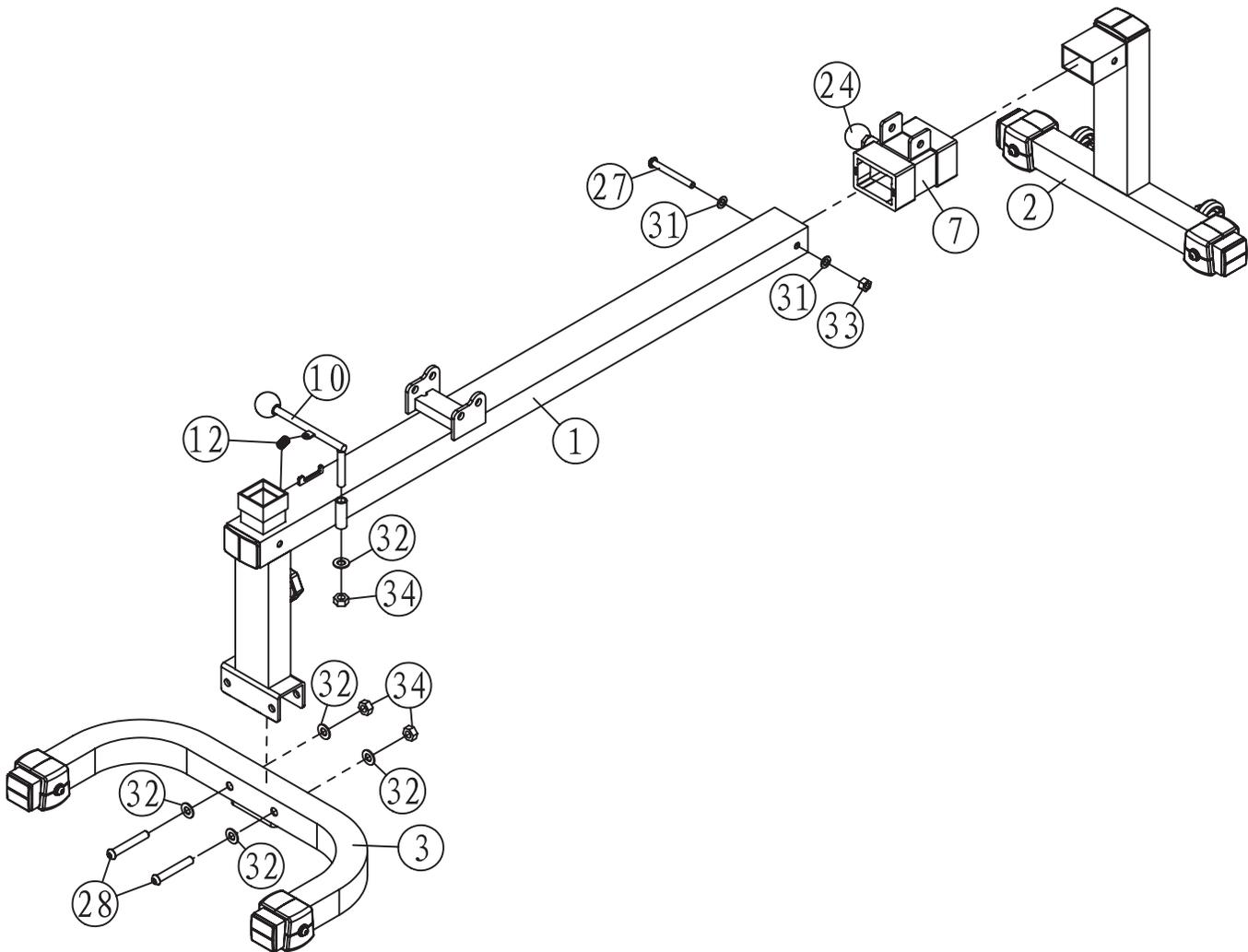
**STEP 1** Connect Main Frame (1) to U-Shaped Base (3) with Bolts (28), Washers (32) and Nylon Lock Nuts (34).
