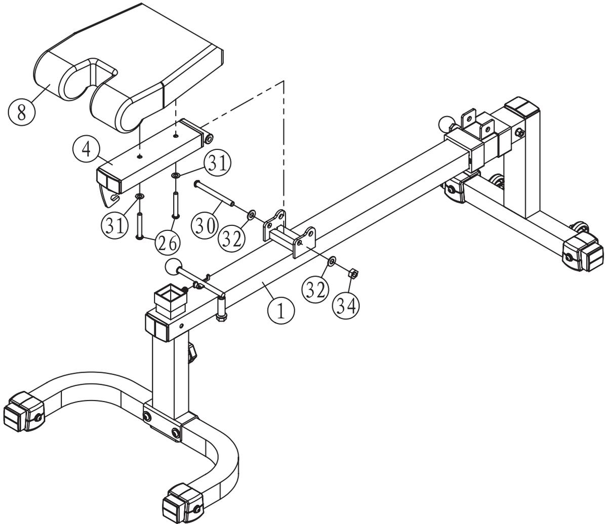
**STEP 2** Connect Seat Pad (8) to Seat Support (4) using Bolts (26) and Washers (31).
