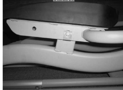
6. Align the hole in the end of the connecting arm (pivoting rod end) with the hole in the bracket of the handle bar. The rod end should be on the inside of the handle bar bracket. Take one of the 1-1/4 X 3/8 bolts and install it through the handle bar bracket and the rod end. Install a flat washer and Nylon nut on the bolt and tighten firmly using a wrench on the nut and one on the bolt.
