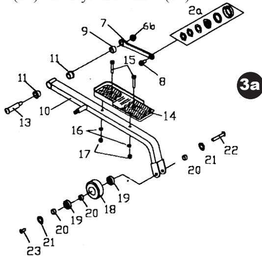
3. Slide the Bolts (12, 13) through the hole of the Foot Pedal Mount Tubes (10) and screw into the Crank (7). Must screw on counter clockwise. Secure both Bolts (12, 13) with Nuts (6a, 6b). Do not forget to place the Plastic Spacer (9) in first. (See 3a above).
