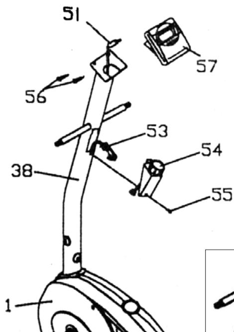
Insert the Tension Knob (54) into the Upright Post (38) and connect with the screw attached (55).
