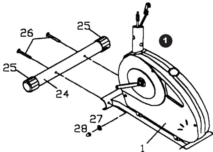
2. Attach the Rear Stabilizer (29) onto the Main Frame (1) using Carriage Screws (26), Cap Nuts (28) and Arc Washers (27).
