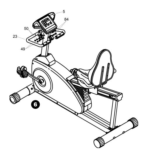
**6.** Attach the pulse wires in the front handlebar (23) to the wires from the console (5). Connect the front handlebar (23) to the console tube with the locknuts (49), flat washers (50) and screws (84) provided. Make sure not to "pinch" any of the pulse wires when connecting the handlebar to the console tube.
