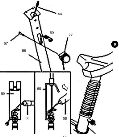
7. Connect the computer cable at the top of the Upright Tube (54) to the Computer (61). Attach the Computer (61) to the Upright Post (56) with the screws attached. Open the battery cover on the back of the computer and install 2 AA batteries.
