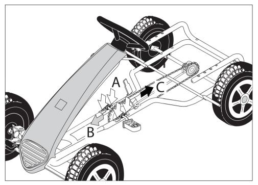
Loosen 4 screws and nuts at location A
