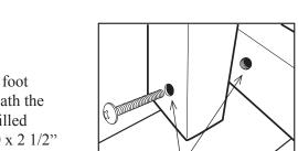
Align the predrilled holes on the leg with the metal insert on the frame, insert the bolt.
