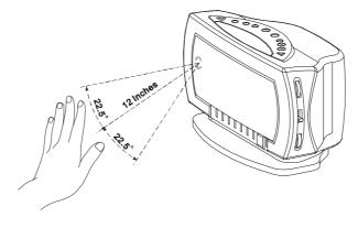
The Touchless Snooze Control works by detecting body heat. For best results your hand should be within 12 inches of the front panel.
