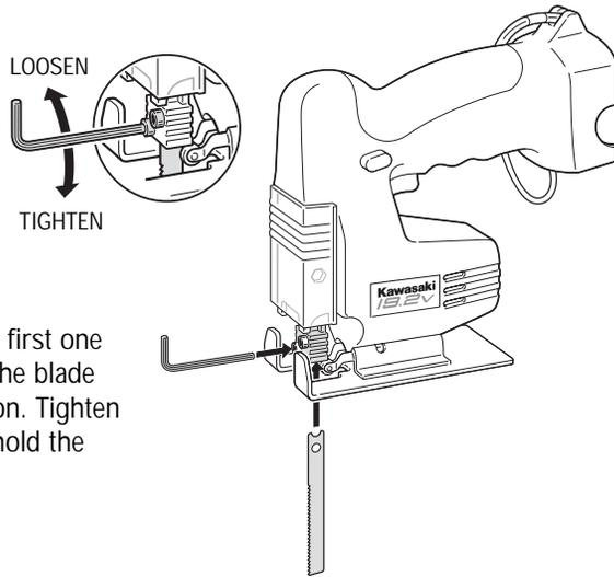
2. Tighten the screws slowly, first one side, then the other, until the blade reaches the desired position. Tighten the screws completely to hold the blade in place.
