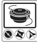
Only use non-metallic, flexible cutting elements, that is trimmer head with trimmer cord.
