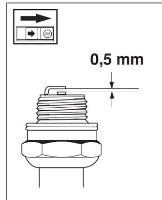
**If the machine is low on power, difficult to start or runs poorly while idling always check the spark plug first.**
