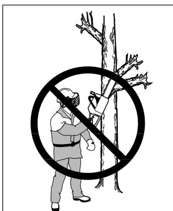
5 In order to keep control of your saw, always maintain a firm foothold. Never work on a ladder, in a tree or on any other insecure support.
