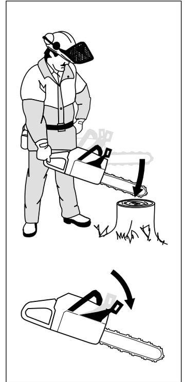
When the bar hits the stump the brake should be applied.
