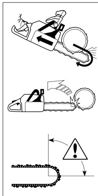
Unless the user resists this pushing force there is a risk that the saw will move so far backwards that only the kickback zone of the bar is in contact with the tree. This will cause kickback.
