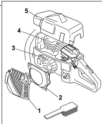
Clean the cooling system with a brush once a week, more often in demanding conditions. **A dirty or blocked cooling system results in the saw overheating which causes damage to piston and cylinder. NOTE! The cooling system of chain saws that are fitted with a catalytic converter must be cleaned daily. This is particularly important on saws with catalytic converters, because the higher working temperature of the exhaust demands efficient cooling of the engine and the catalytic converter unit.**
