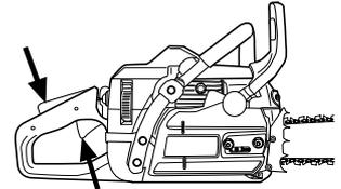
CAUTION! Do not release the starter handle from fully pulled out position as this can cause damage on the saw.
