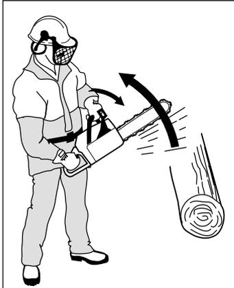
If the kickback is less violent or the kickback zone of the bar is closer to you the chain brake will be activated manually by the movement of your left hand.
