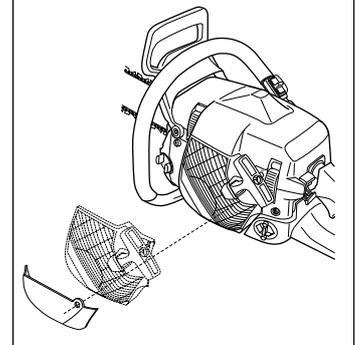
**IMPORTANT!** If the temperature rises above -5°C (23°F) or 0°C (32°F) respectively the saw **MUST** be restored to its normal settings. Otherwise there is a risk of overheating, which can cause severe engine damage.
