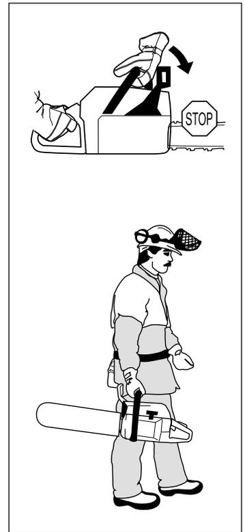
b You can also use the chain brake as a temporary brake when you change position or if you put the saw down for a short time. You should also apply the chain brake manually if there is a risk of the chain accidentally hitting anyone or anything close by.
