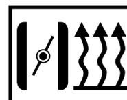
If your saw bears this decal it is equipped with carburettor heating.
