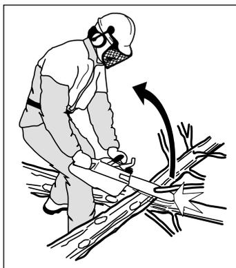
4 Never use the saw above shoulder height and try not to cut with the tip of the bar.
