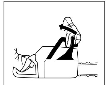
5 As mentioned in section A, kickback can be very sudden and violent. **Most kickbacks are minor and do not always activate the chain brake. If this happens you should hold the chain saw firmly and not let go.**
