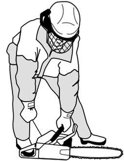
Push in the choke control immediately when the engine ignites and make repeated starting attempts. When the engine starts, rapidly give full throttle. Then the throttle latch will disengage.
