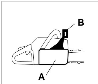
The brake is applied when the front hand guard (B) is pushed forwards.
