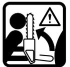
Tip contact may cause the guide bar to move suddenly upward and backward, which may cause serious injury. Please see pages 12-21 in your "Chain saw operator's safety manual".
