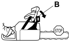
This movement activates a spring-loaded mechanism that tightens the Brake Band (C) around the engine drive system (D) (Clutch Drum).
