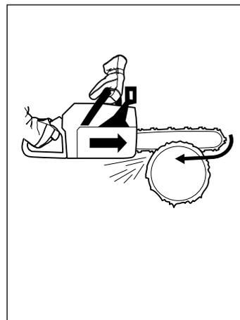
In this case the saw pulls itself towards the tree and the front edge of the saw provides a natural rest when cutting. Cutting on the pull stroke gives you better control over the saw and the position of the kickback zone.
