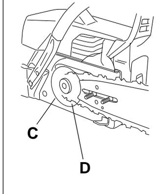
2 The front hand guard is not designed solely to activate the chain brake. Another important safety feature is that it prevents the chain from hitting your left hand if you lose your grip on the front handle.
