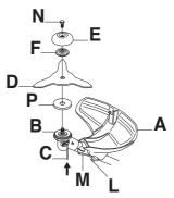
Screw the support cup (E) onto the output shaft threads (CAUTION! Left-hand thread). Tighten to a torque of 35-50 Nm (3.5-5.0 kpm). Use the socket spanner in the tool kit. Note that the locking pin (C) must remain inside the gear housing to lock the drive disk. Hold the shaft of the socket spanner as close to the blade guard/combination guard as possible.
