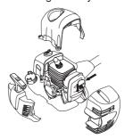
Some mufflers are equipped with a special spark arrestor screen. If your machine has this type of muffler, you should clean the screen at least once a week. This is best done with a wire brush.
