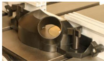
The POWERMATIC 18" Drill Press comes with a 2 3/4"-tall by 19 3/4"-wide fence. The fence has a pair of flat, extruded aluminum faces that can be opened to increase the overall support to 30"! Splitting the fence faces also reveals the inlet for the built-in dust collection that terminates in a 2"-diameter ID (2 1/4" OD) port that angles out from the rear of the fence
