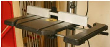
We opened just the right table wing to show the dramatic difference these sliding wings offer. When working with large stock pieces, the PM2800 handles the job with ease.
