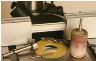
With the fence faces opened (left) the built-in dust port is revealed. The one-piece aluminum dust port and fence bracket (right) make aligning the PM2800 fence system easy and very precise.
