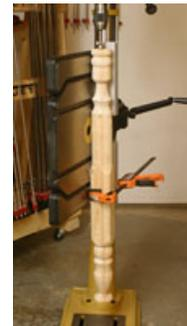
The table can also be tilted to 90-degrees to the left or right for working with long pieces. While tilted the table can still be moved left, right, up and down.
