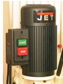
The 1 Hp motor and easy to use switch provides the power and control you need.
