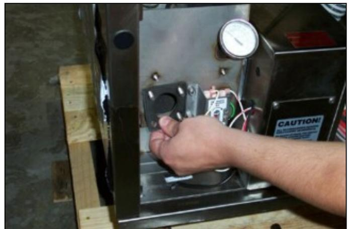
Removing the heater gasket
