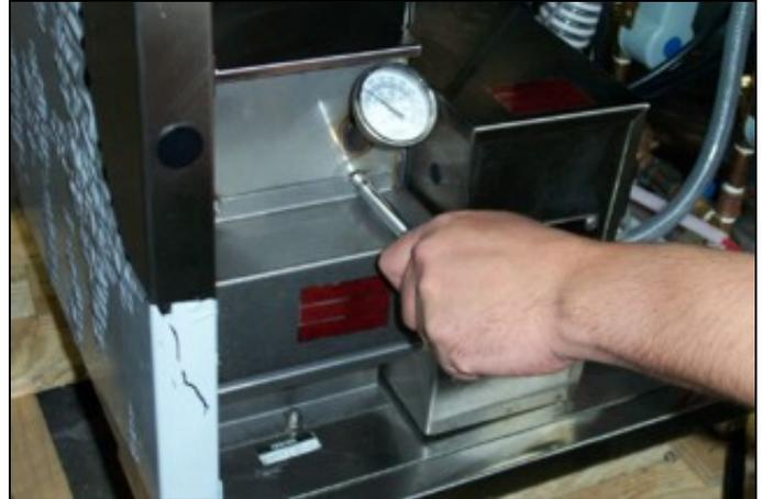
Removing the heater cover.
