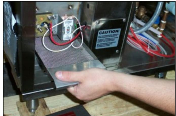
Removing the lower strainer.
