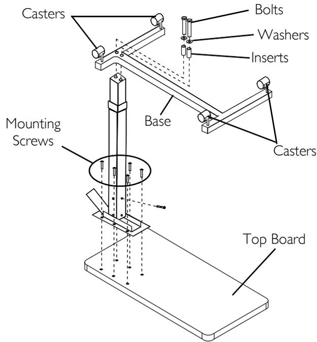
**FIGURE 1** Assembling the Overbed Table - Model 6417
