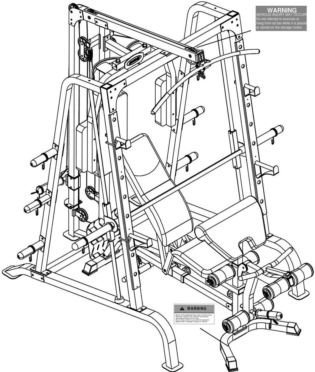
The warning labels shown here have been placed on the Front Stabilizer and Upper Frame. If the labels are missing or illegible, please call customer service at 1-800-888-8899 for replacements. Apply the labels in the location shown.
