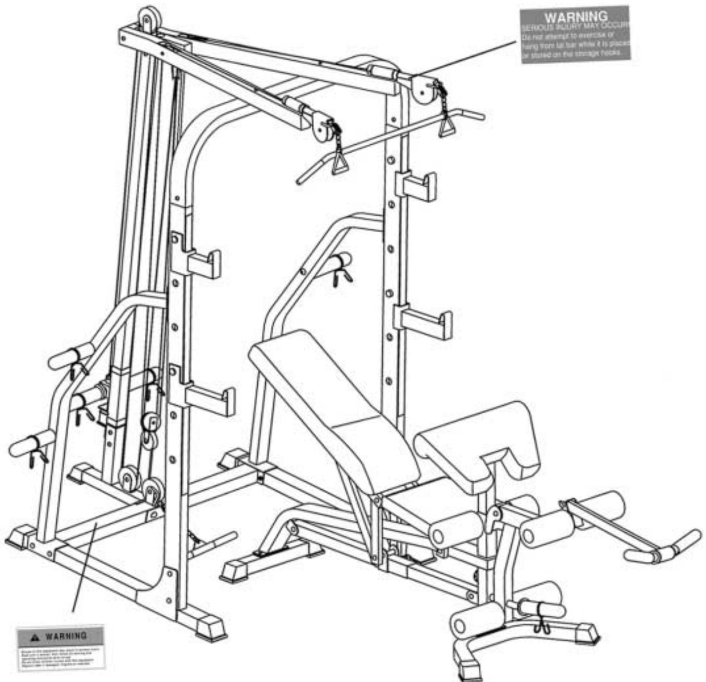
The warning labels shown here have been placed on the Rear Base and Upper Frame. If the labels are missing or illegible, please call customer service at 1-800-888-8899 for replacements. Apply the labels in location shown.
