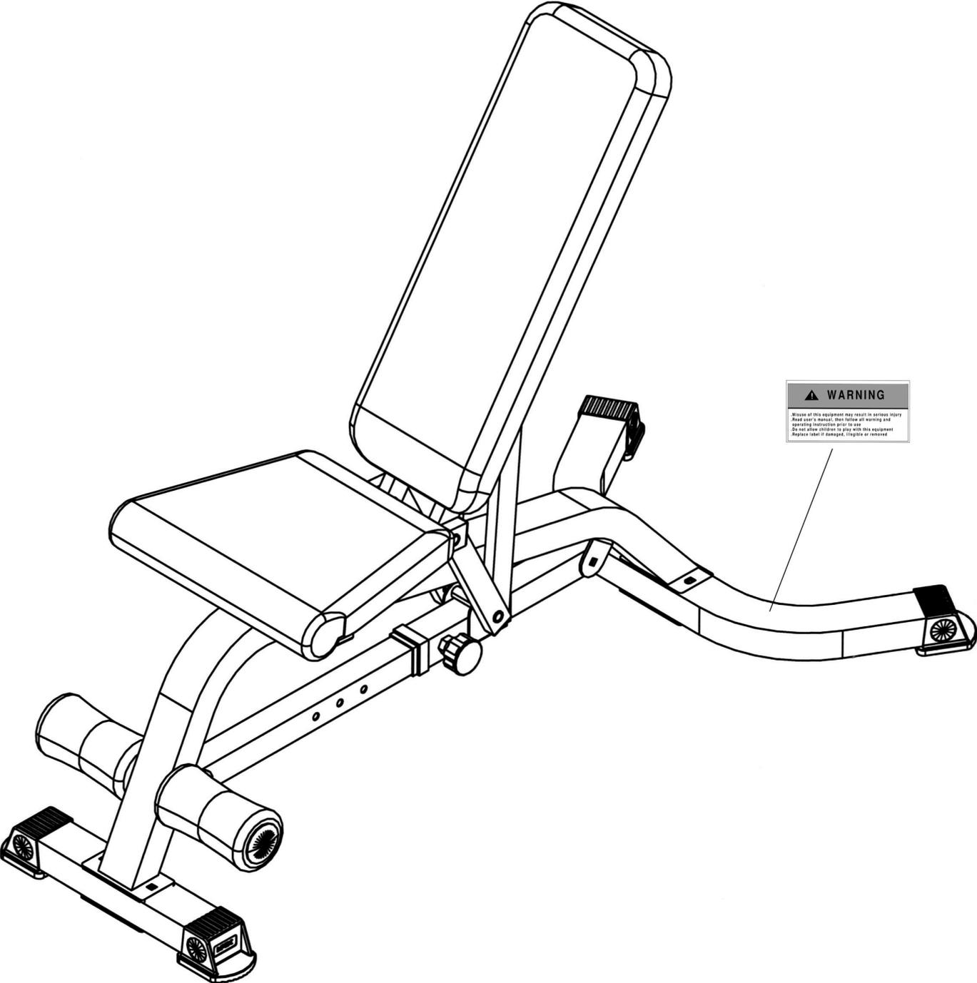
The Warning Label shown here has been placed on the Rear Base. If the label is missing or illegible, please call customer service at 1-800-999-8899 for replacement. Apply the label in the location shown.
