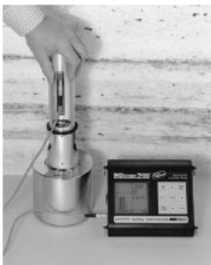
Fig. 6.1 Performance check of the concrete test hammer
