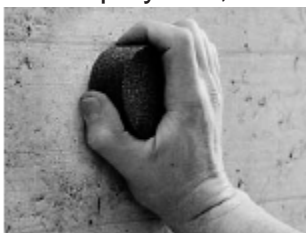
Fig. 5.1 Preparing the test surface
