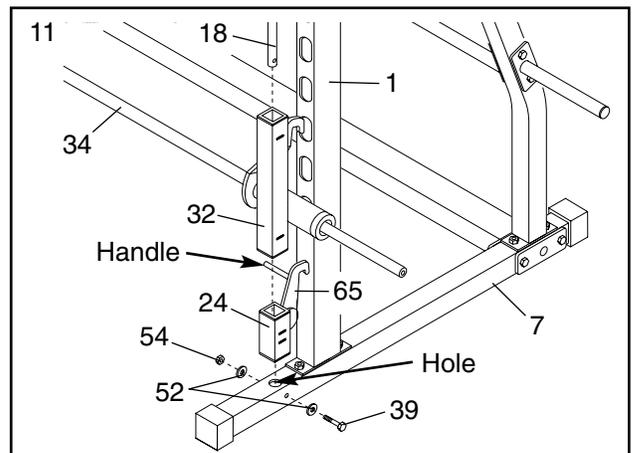
12. Place the Right Safety Spotter (23) on the right Base (7) and center it over the indicated hole. **Note: The handle must point toward the center of the bench.**
