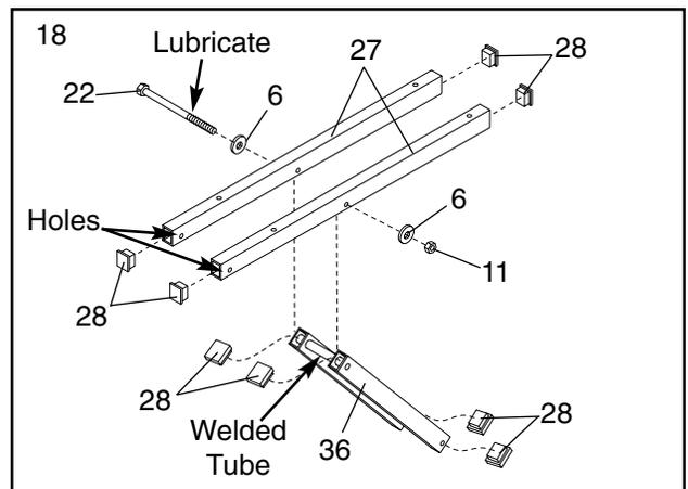
19. Lubricate an M10 x 115mm Bolt (55). Slide an M10 Washer (6) onto the Bolt.
