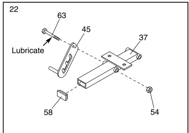
23. Place the Seat Support Tube (37) on the Bench Frame (5) so that the Seat Adjustment Bracket (45) fits over the welded pin (not visible in the drawing) on the side of the Bench Frame.
