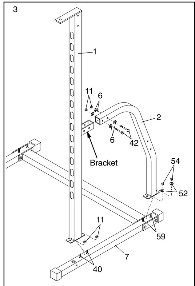
4. Slide the remaining Brace (2) onto the bracket on the other Upright (1). Attach the Brace to the Upright with two M10 x 65mm Bolts (42), four M10 Washers (6), and two M10 Nylon Locknuts (11). **Do not tighten the Nylon Locknuts yet.**
