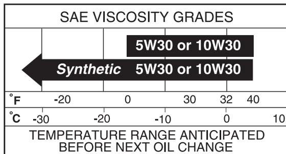
**NOTE:** Although multi-viscosity oils (5W30, 10W30 etc.) improve starting in cold weather, these multi-viscosity oils will result in increased oil consumption when used above 32°F. Check your engine oil level more frequently to avoid possible engine damage from running low on oil.
