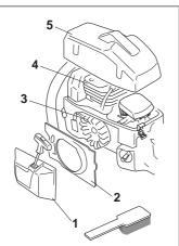
Clean the cooling system with a brush once a week, more often in demanding conditions. A dirty or blocked cooling system results in the saw overheating which causes damage to piston and cylinder.
