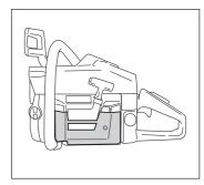
NOTE! If the special winterising kit has been fitted or any measures have been taken to increase the temperature these changes must be reversed before the saw is used in normal temperature conditions. Otherwise there is a risk that the saw will overheat, resulting in severe damage to the engine.
