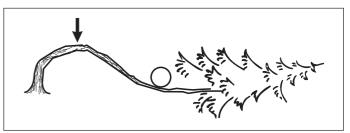
b) Decide which is the SAFEST way to release the tension and whether YOU are able to do it safely. In complicated situations the only safe method is to put aside your chain saw and use a winch.
