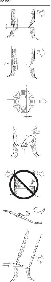
We recommend that you use a bar that is longer than the diameter of the tree, so that you can make the FELLING CUT and DIRECTIONAL CUT with single cutting stokes. (See *"Technical data"* to find out which lengths of bar are recommended for your saw).
