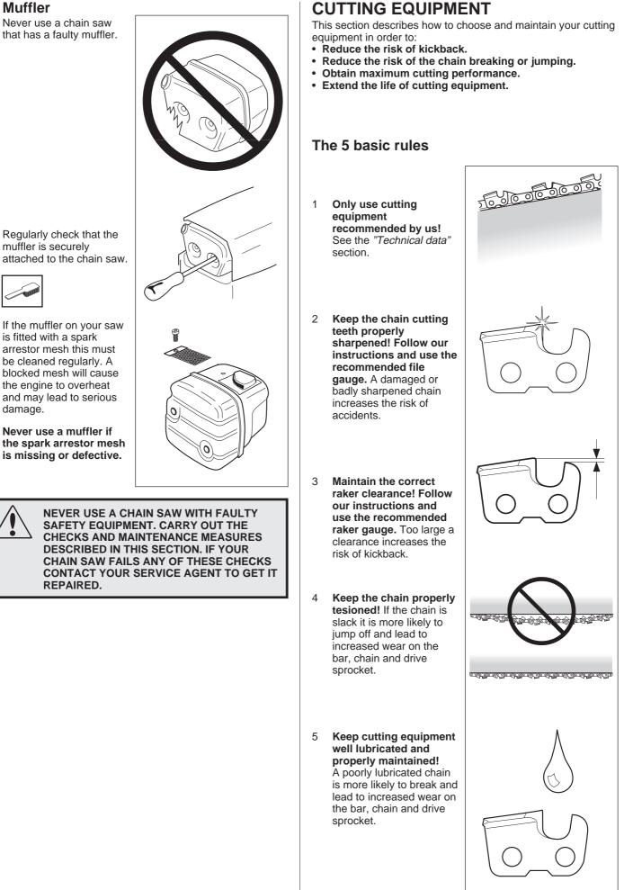
muffler is securely attached to the chain saw.
