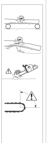
Two factors decide whether the chain will jam or the log will split. The first is how the log is supported and the second is whether it is in tension.
