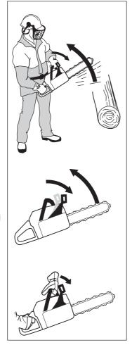
7 During felling your left hand grasps the front handle in such a way that it cannot activate the front hand guard. In this position the chain brake can only be activated by the inertia action of the counterweight.
