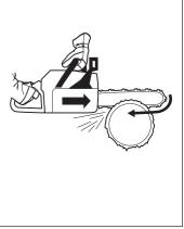
7 Follow the instructions on sharpening and maintaining your bar and chain. When you replace the bar and chain use only combinations that are recommended by us. See the sections on *"Cutting equipment"* and *"Technical data"*.
