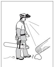
5 Take the utmost care when cutting through branches or logs that are in tension. A log or branch that is in tension can suddenly spring back into its natural position before or after you cut it. If you stand on the wrong side or start cutting in the wrong place it may strike you or your chain saw. This could make you lose control and cause a serious accident.
