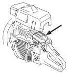
The filter can be cleaned more thoroughly by washing it in water and detergent.
