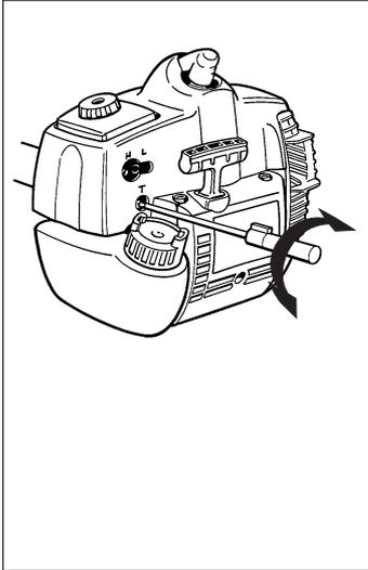
**CAUTION!** Contact your servicing dealer, if the idle speed setting cannot be adjusted so that the cutting attachment stops. Do not use the machine until it has been properly adjusted or repaired.
