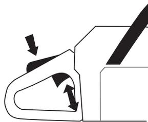
4 Start the saw and apply full throttle. Release the throttle control and check that the chain stops and remains stationary. If the chain rotates when the throttle is on idle setting you should check the carburetor idle adjustment. See the section on "Maintenance".
