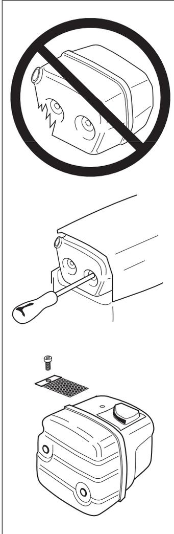
Regularly check that the muffler is securely attached to the chain saw.
