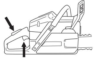
CAUTION! Do not release the starter handle from fully pulled out position as this can cause damage on the saw.
