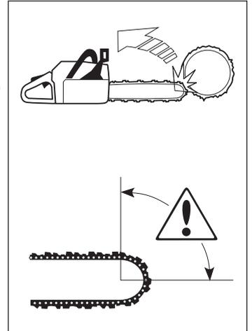
Kickback always occurs in the cutting plane of the saw. Normally the saw and bar are thrown backwards and upwards towards the user. However the saw may move in a different direction depending on the way it was being used when the kickback zone of the bar touched the object.
