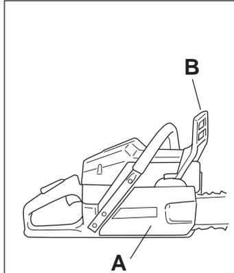
The brake is applied when the front hand guard (B) is pushed forwards.
