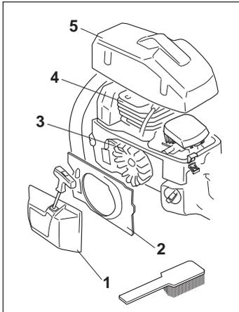
Clean the cooling system with a brush once a week, more often in demanding conditions. **A dirty or blocked cooling system results in the saw overheating which causes damage to piston and cylinder.**
